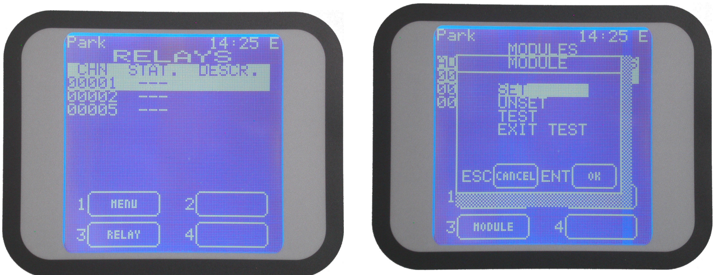
Figure 37 Outputs screen and options available pressing 3-Relay
