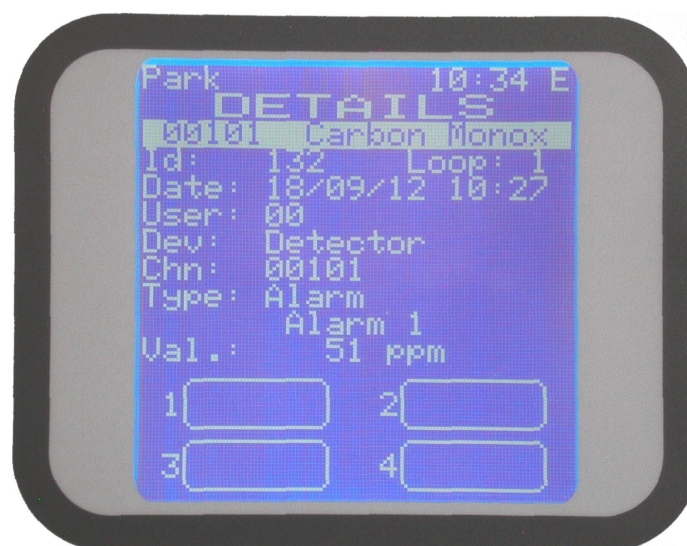
Figure 22 ALARM details screen.
