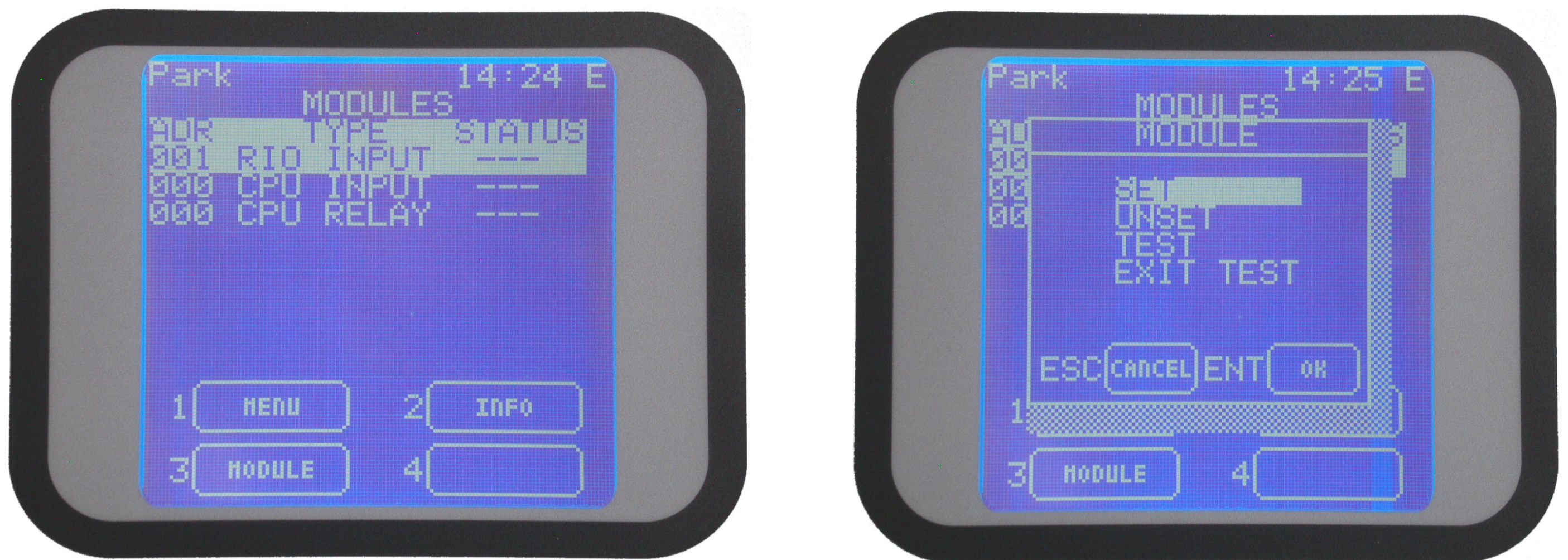
Figure 36 Modules screen and available options pressing 3-Module
