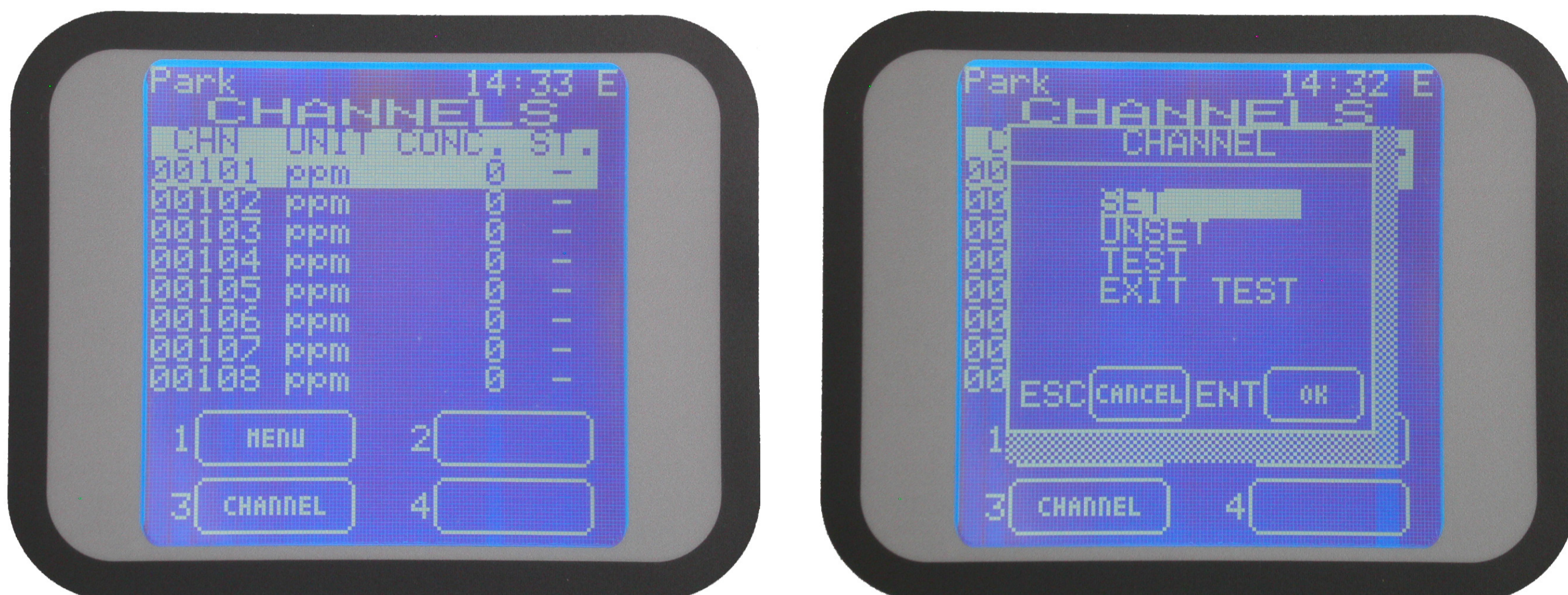
Figure 40 Detectors screen and options available pressing 3-Channel
